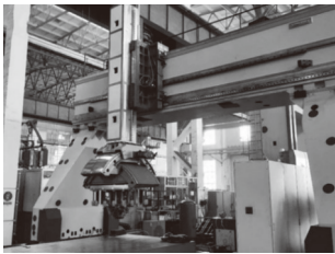
图5 通用技术齐二机床地轨龙门式碳纤维复合材料铺丝/铺带设备 Fig. 5 Ground rail gantry-type AFP equipment developed by Qiqihar No.2 Machine Tool (Group) Co., Ltd.
